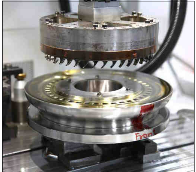
ISRO Crio Engine Rotor Machining
